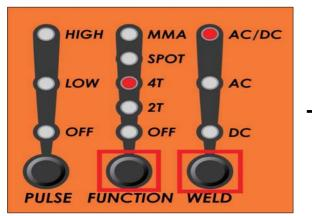
1) Select the AC/DC by pressing the weld button. Then, select the 4T by pressing the function button.
