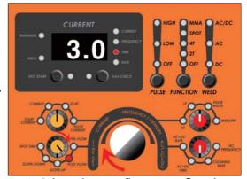
4) Select the pre-flow, post-flow by turning the time set knob. Then, set 0.2, 3 sec each by control volume.
