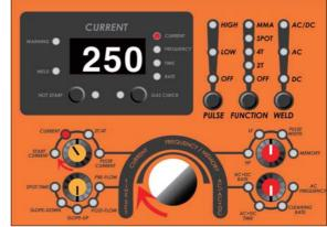
2) select the current by turning the current knob. Then, set the 250A by the control volume.
