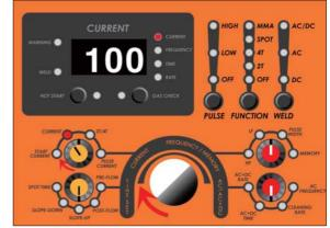
2) Select the current by turning the current knob. Then, set the 100A by the control volume.
