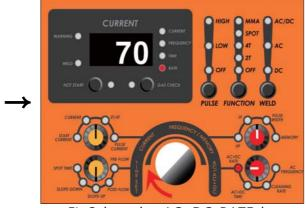
5) Select the AC+DC RATE by turning the AC/AC+DC knob. Then, set 70% by control volume.
