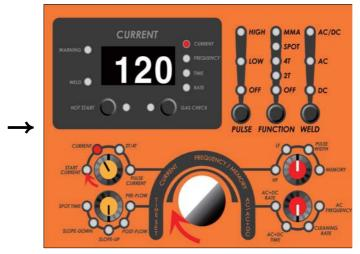
3) Select the welding current by using the current knob. Then, adjust the current properly.
