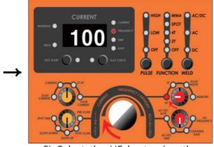
5) Select the HF by turning the frequency / memory knob. Then, set 100Hz by control volume.
