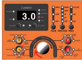
4) Select the post-flow by turning the time set knob. Then, set 3 sec by control volume.
