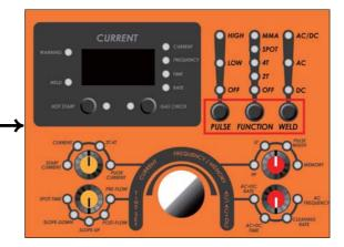
4) Set the welding condition by using pulse button, function button, welding button.
