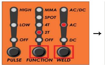
1) Select the AC by pressing the weld button. Then, select the 2T by pressing the function button.
